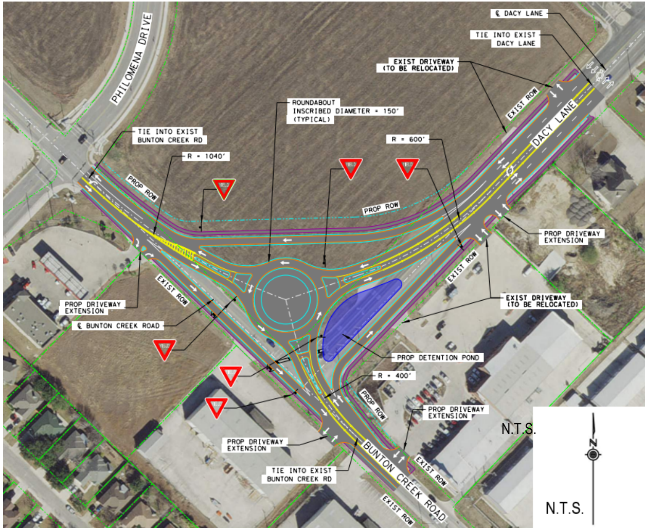
Figure 5.1: Preliminary Roundabout Layout
