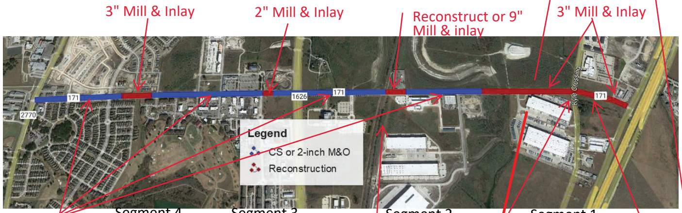
Figure 44. Repair Recommendations for WB Direction
