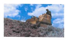
We are also the designer and exclusive manufacturer of the SUTTER 300 Mini Trail Dozer™ (U.S. patent D785,680), a 30 inch wide, 4,300 lb. trail machine used to build and maintain "single-track" trails.
