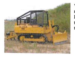
We are the original designer of the Trail Dozer<sup>TM</sup> and the exclusive manufacturer of the SUTTER 500 Trail Dozer<sup>TM</sup>, a 48 inch wide, 9,000 lb. trail machine used to build and maintain 3 to 4 foot wide trails, and has the maneuverability to get into tight places for thinning or removal of trees in the forest, etc.
