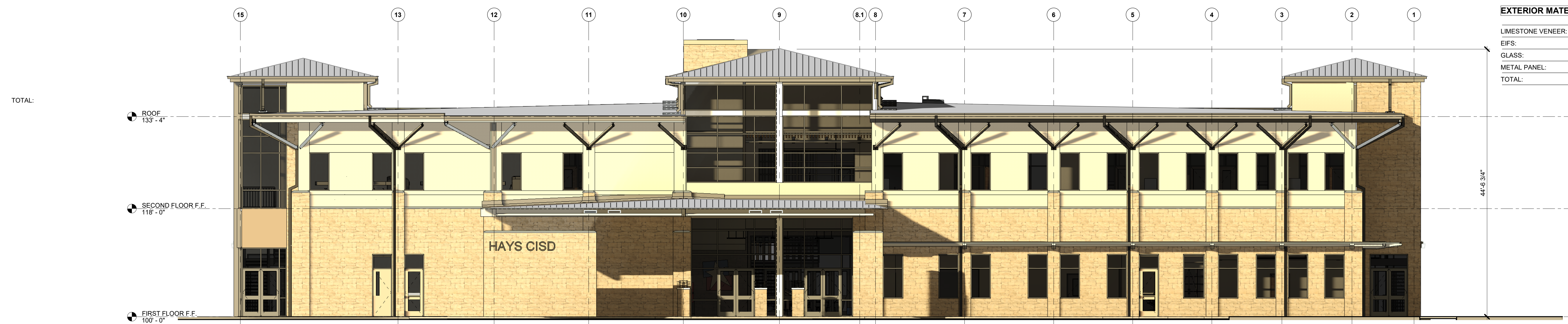
1 CONCEPTUAL EAST ELEVATION (FRONT) SCALE: 1/8" = 1'-0"
