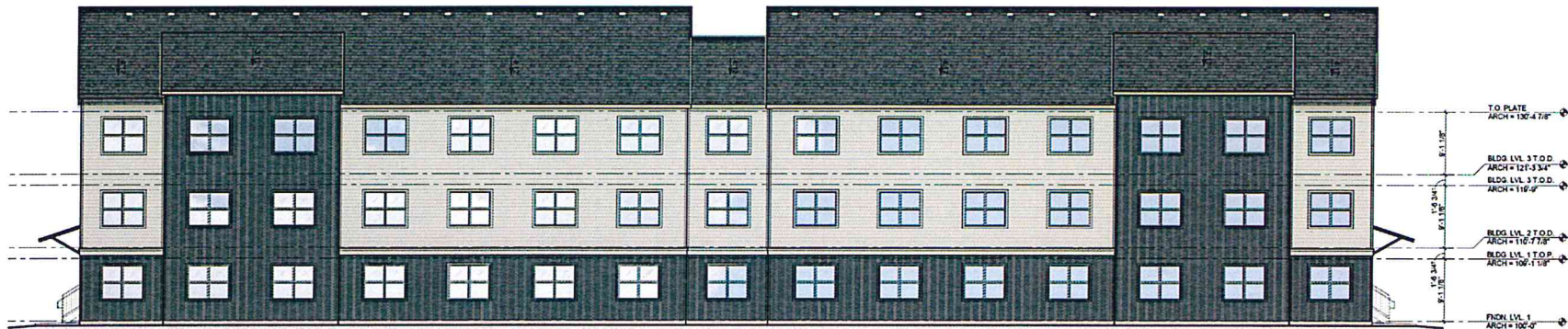
02 BUILDING TYPE I - REAR ELEVATION SCALE: 1/16" = 1'-0"
