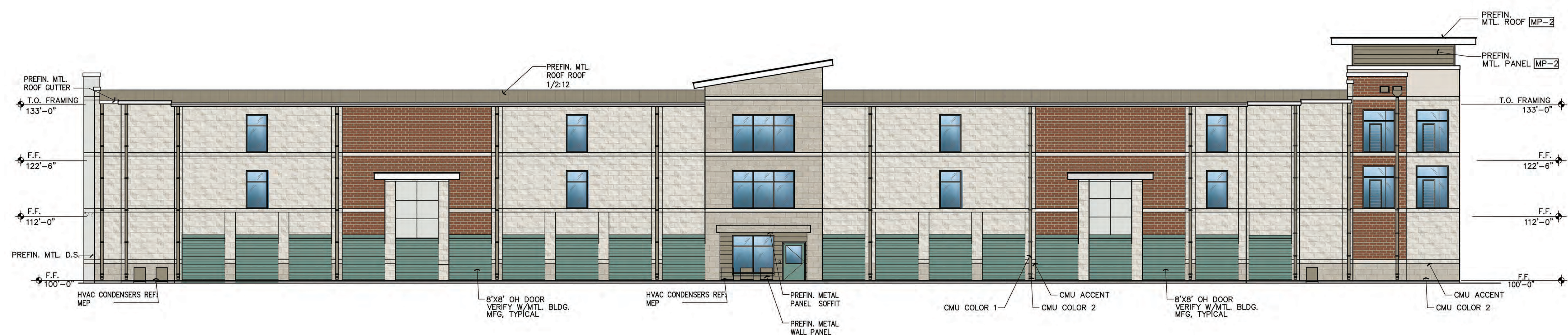
02 NORTH ELEVATION - BUILDING "B" SCALE: 1" = 10'-0"
